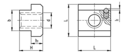
b -0.1 -0.3 = 10 d = M8 H = 12 h1 = 6 L = 15 I1 = 0.7 T-slot width DIN 650 = 10 Weight (g) = 14
